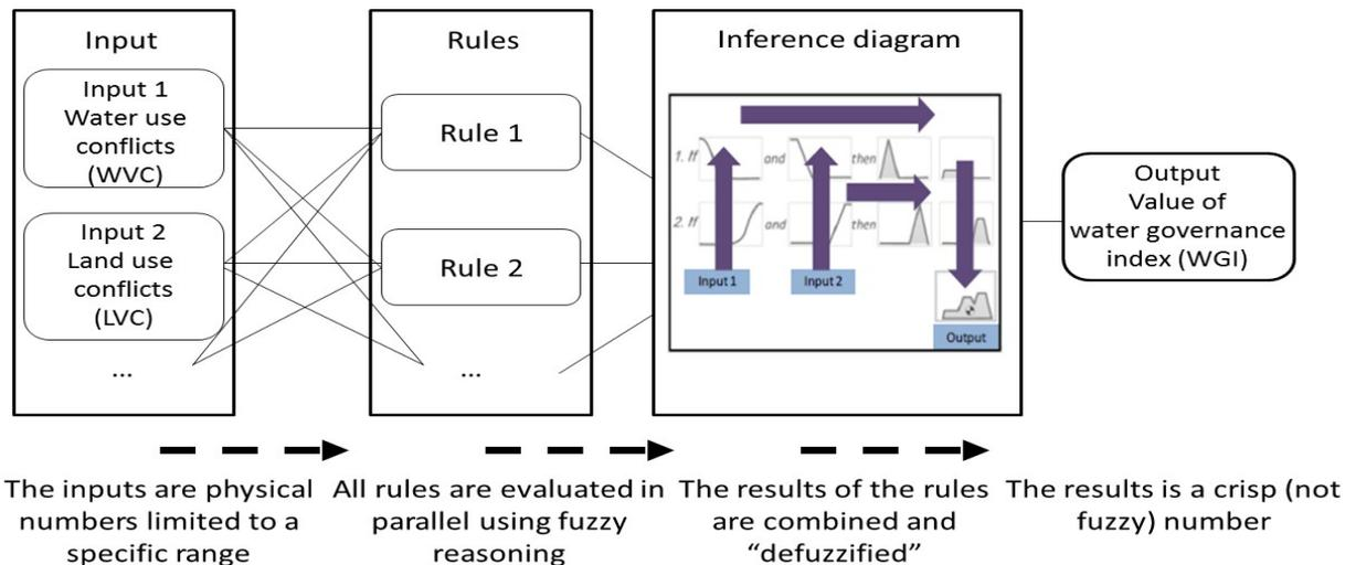
**Figure 2. Overview of the fuzzy inference process (Adapted from Jia et al., 2016: 5).**
