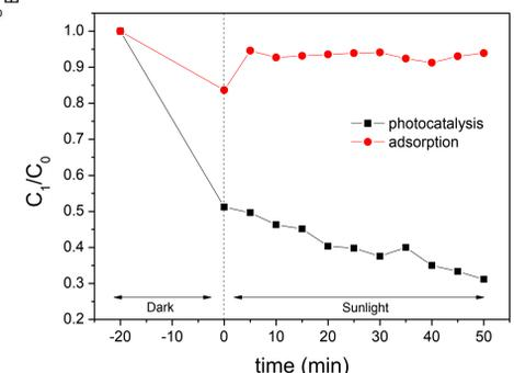
Figure 04. Photocatalysis and adsorption the Bent 250 under solar irradiation.
