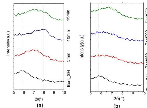
Figure 02. XRD spectra CdS/Bent varying the reaction time (a) and proportion the bentonite (b).
