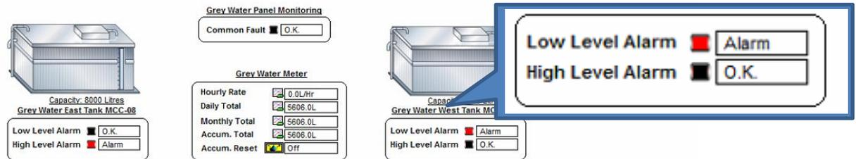
Figure 5: Header tanks fault shown on BMS GUI.
