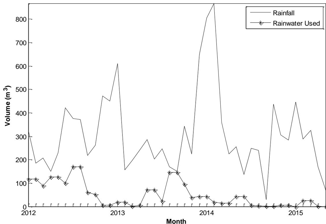
Figure 4: Quantity of rainfall and rainwater pumped to header tanks per month, 2012-2015.
