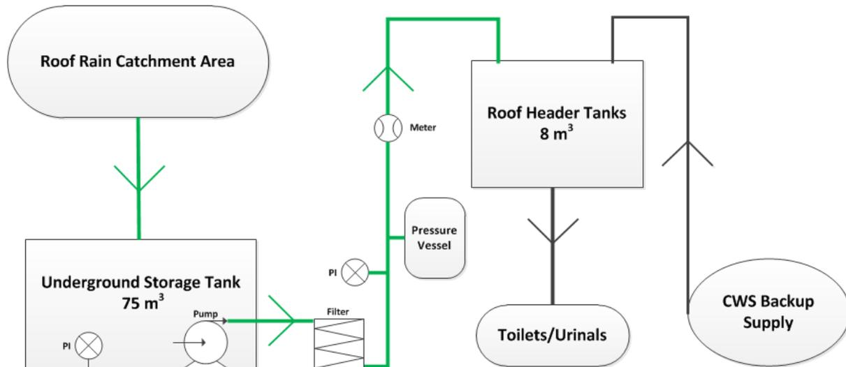
Figure 3: Schematic representation of the NUI Galway engineering building RWHS
