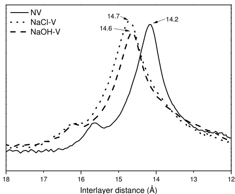
Fig. 1 – Increase on interlayer distance after sodium chloride (NaCl-V) and sodium hydroxide (NaOH-V) treatments.
