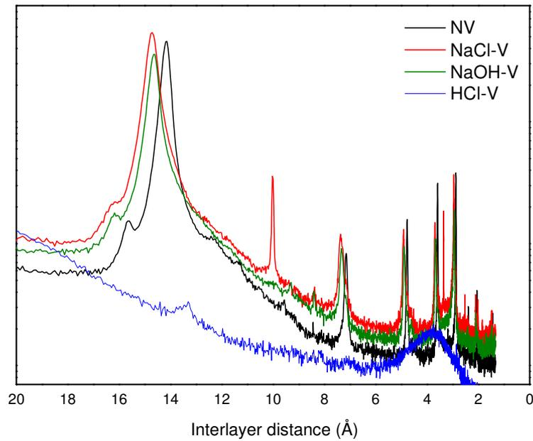
Fig. 2 – X-ray diffractograms of vermiculite samples, showing structural disorder of hydrochloric acid treated vermiculite (HCl-V).
