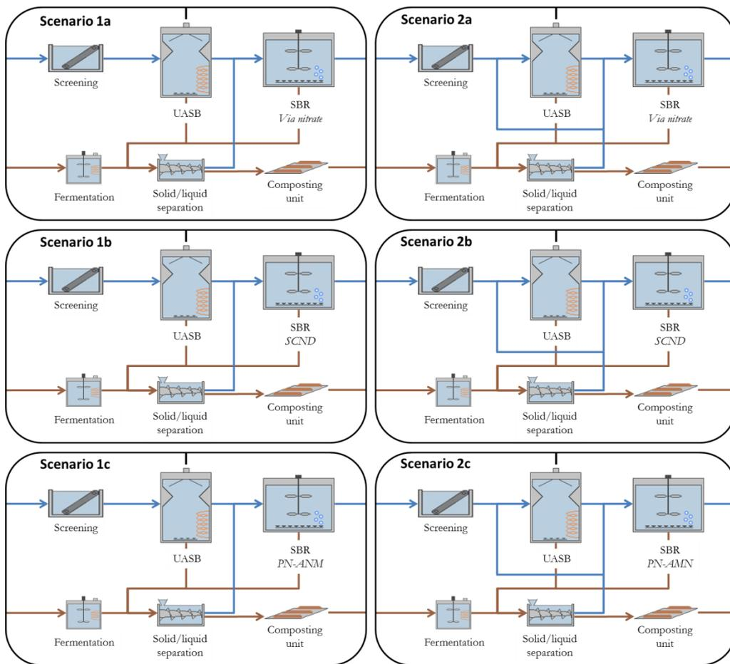
**Figure 2.** Alternative scenarios focusing on nitrogen removal with and without recirculation of the fermented liquid into the anaerobic treatment unit.
