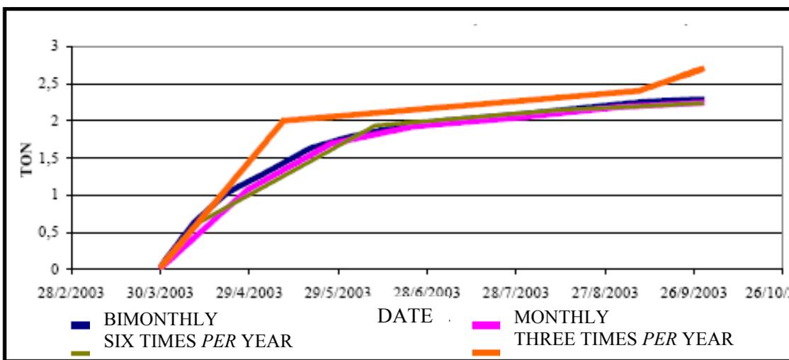
**Figure 04 – Load of phosphorus during the dry period, at the exit of the Descoberto Reservatory.**
