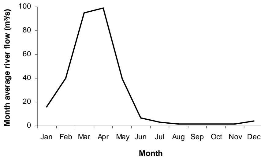
Figure 2. Monthly average river discharge in the Icó section (1957-2005)
