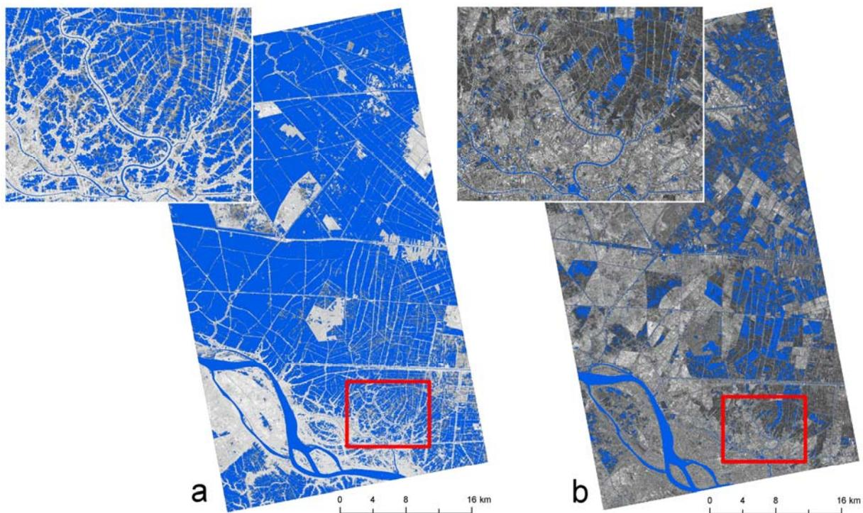
**Figure 3: The SAR images from October 20<sup>th</sup> 2007 (a) and January 5<sup>th</sup> 2008 (b) superimposed with the derived watermasks. The zoomed images show the high detail of the sensor and the derived results and the rate of change in both images.**
