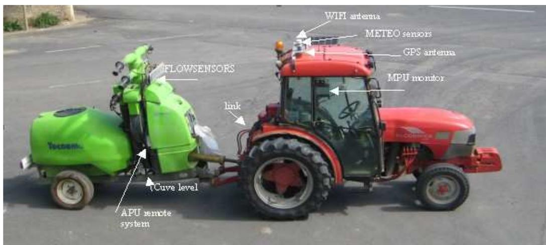
Fig 3: the implementation of the Aware device on the Cemagref tractor.
