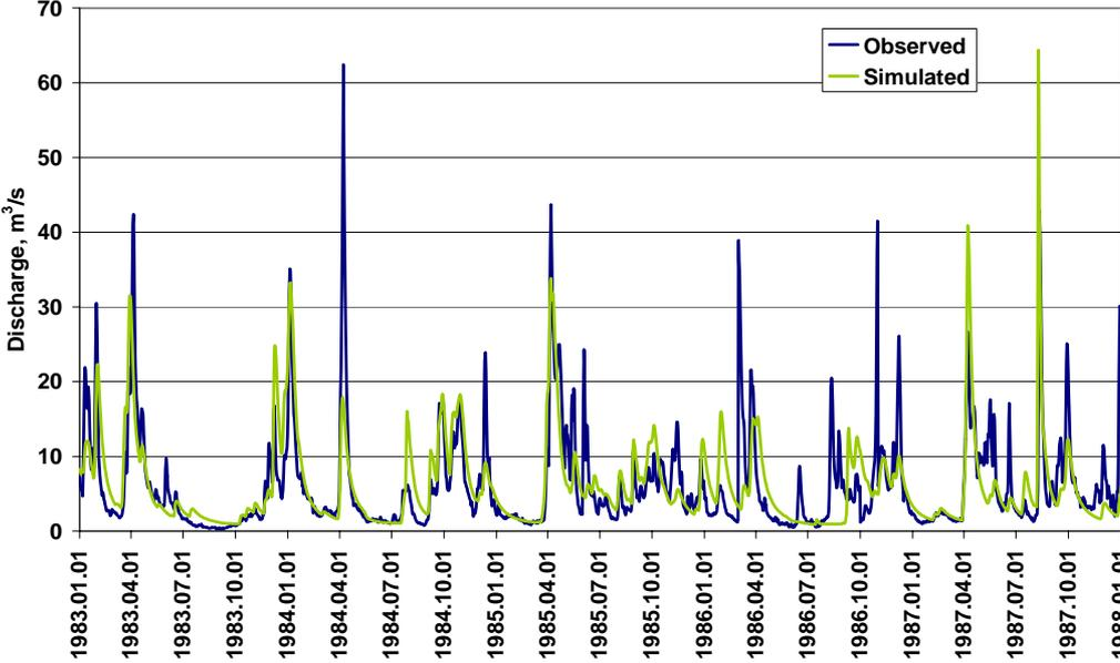
Figure 4 Observed and simulated daily discharge at runoff gauge Rūja-Vilnīši
