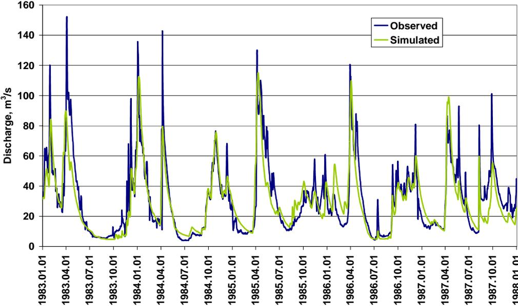
Figure 3 Observed and simulated daily discharge at runoff gauge Salaca-Lagaste
