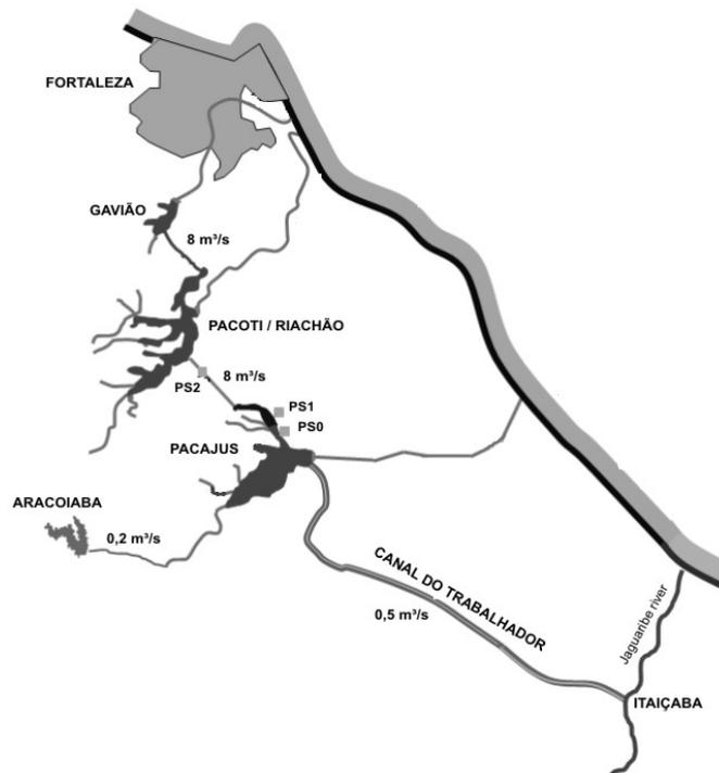
**Figure 1: Current reservoirs' system used for water supply of the metropolitan region of Fortaleza. The system consists of 5 reservoirs and 3 pumping stations. The *Canal do Trabalhador* diverts water from the Jaguaribe River Basin, near the city of Itaipaba into the Pacajus reservoir.**
