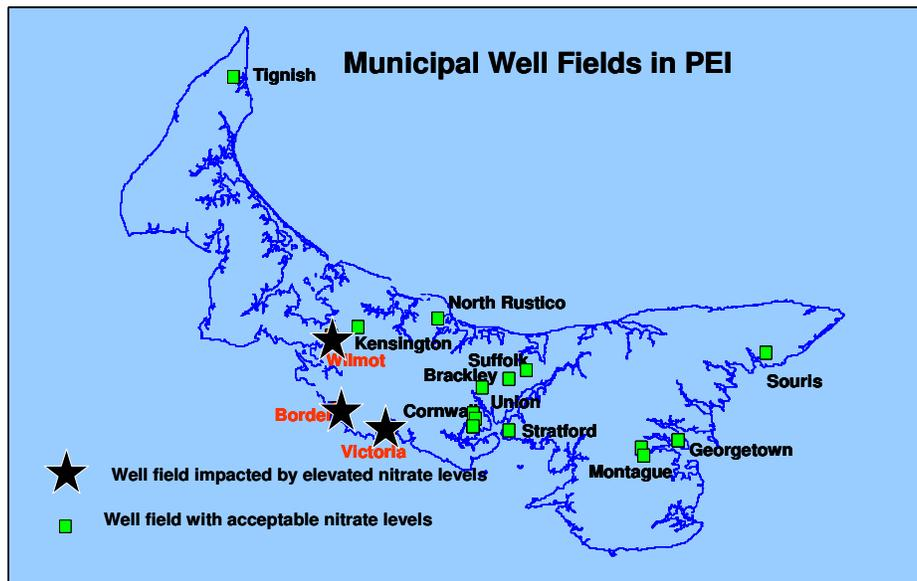
**Figure 4.** Municipal water supply utilities in PEI, with well fields impacted by elevated nitrate levels indicated by stars.
