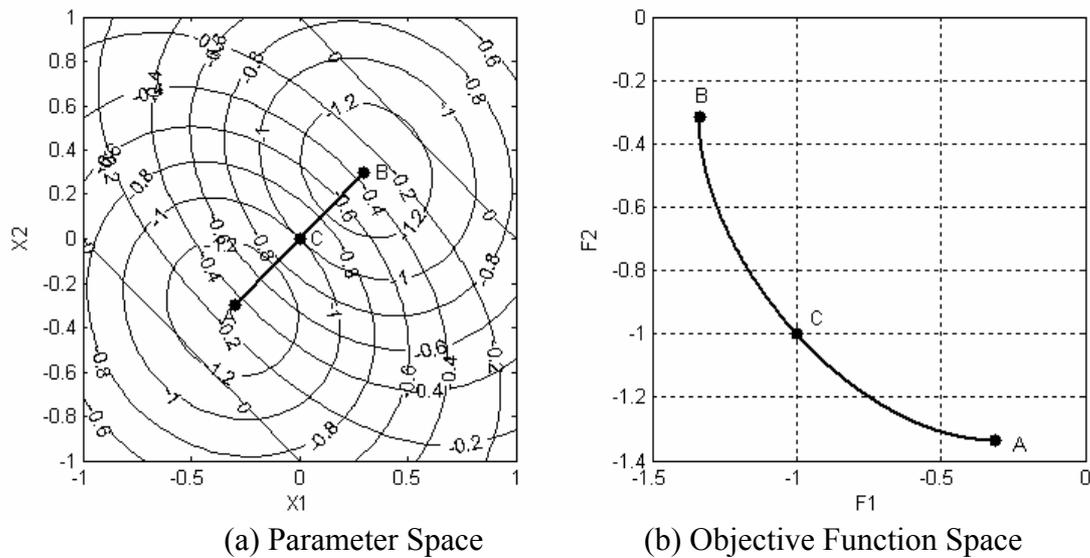
Figure 1 – Illustration of the Pareto optimal solution concept for a minimization problem with two objectives (F1, F2) in a search space ( $\Delta\delta$ ) bi-parametric ( $\theta_1, \theta_2$ ): a. parametric space; b. functions space (Vrugt et al., 2003).
