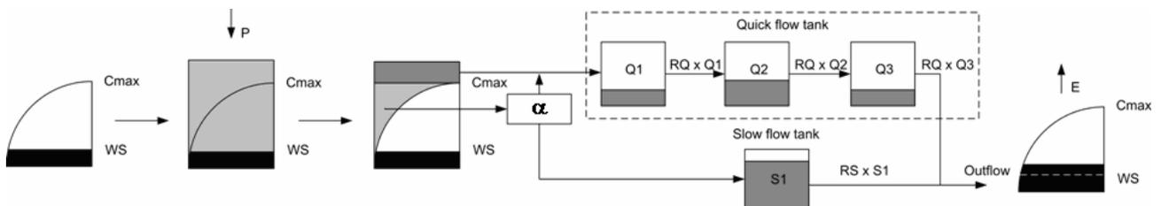
Figure 3 – Schematic representation of the hydrologic model HYMOD.
