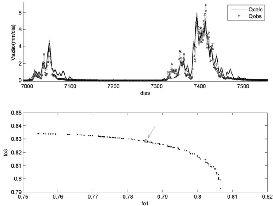
Figure 6 – Observed hydrograph and optimal hydrographs associated to Pareto Front points for the objective functions  $OF_1$  and  $OF_3$ . Dotted line represents the observed hydrograph while the continuous line represents the solution correspondent to the point of the Pareto Front indicated by the arrow (Hydrographs associated to other points in the Pareto Front are represented by grey lines). The identified Pareto Front is presented below the hydrographs.
