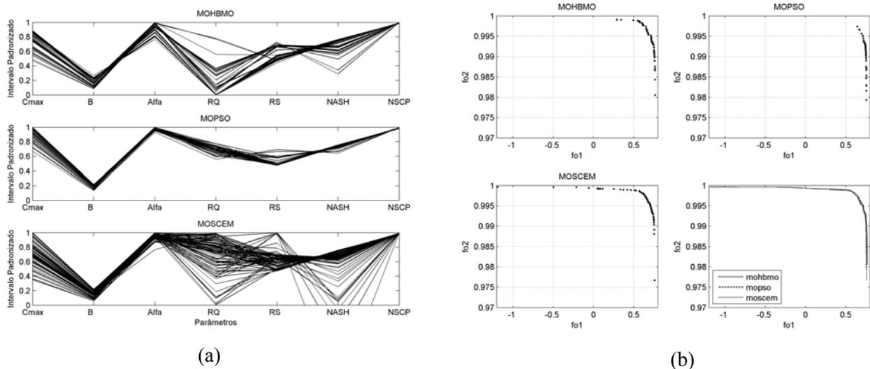
Figure 5 – Optimum solutions identified by the algorithms MOHBMO, MOSCEM and MOPSO using OFs 1 and 2 in the calibration of the model HYMOD for the stream gage station 34750000: (a) Set of optimal parameters; (b) Identified Pareto Fronts.
