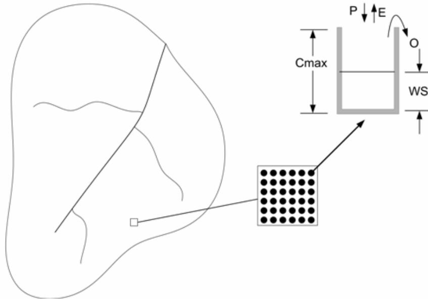
Figure 2 – Watershed representation in the HYMOD model (P: Precipitation; E: Evaporation; O: Outflow; WS: Water Storage;  $C_{max}$  is the largest water storage capacity within the watershed).
