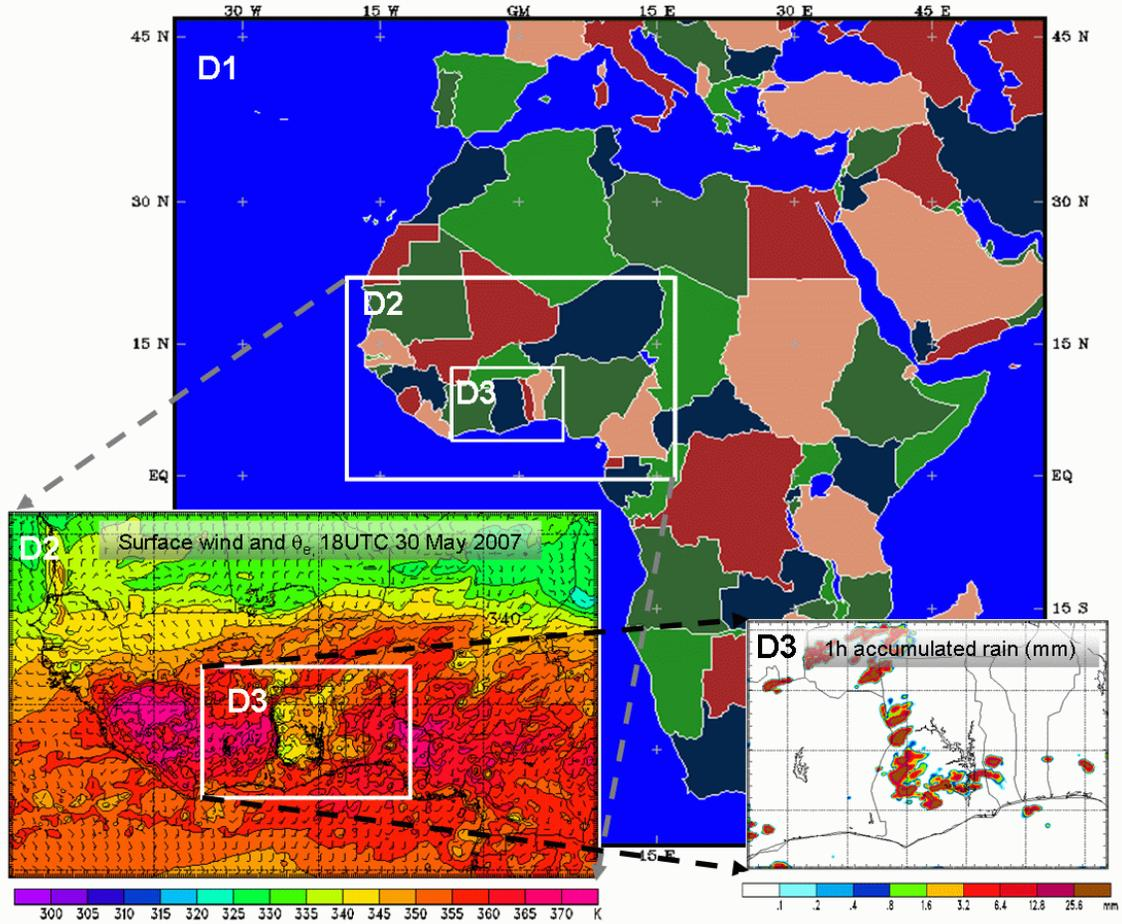
**Figure 2.** WRF forecast domains for the operational modeling system, with example forecast products on the two inner grids. The grid increments on D1, D2, and D3 are 40.5, 13.5 and 4.5 km, respectively. The forecasts are 48 h in duration on D1 and D2, and 36 h on D3.
