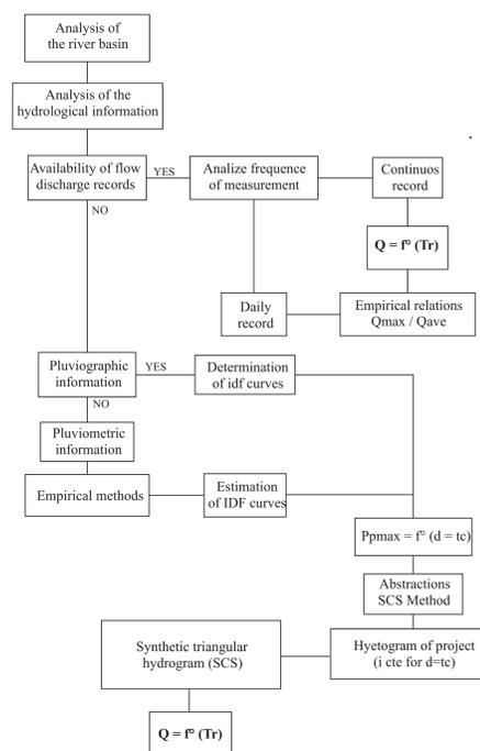
Figure 4 - Hydrological estimations for a basic project
