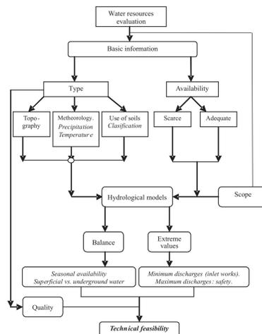
Figure 2 - Superficial flow determination
