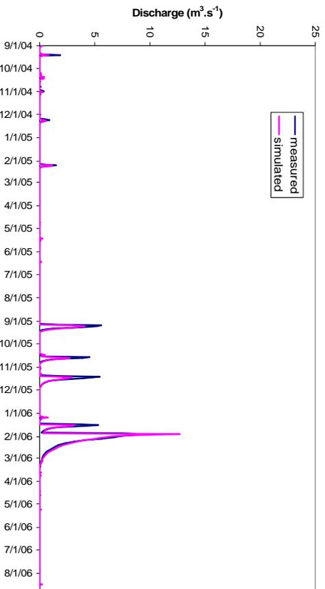
Fig. 4 Simulated and measured hydrographs for the validation period
