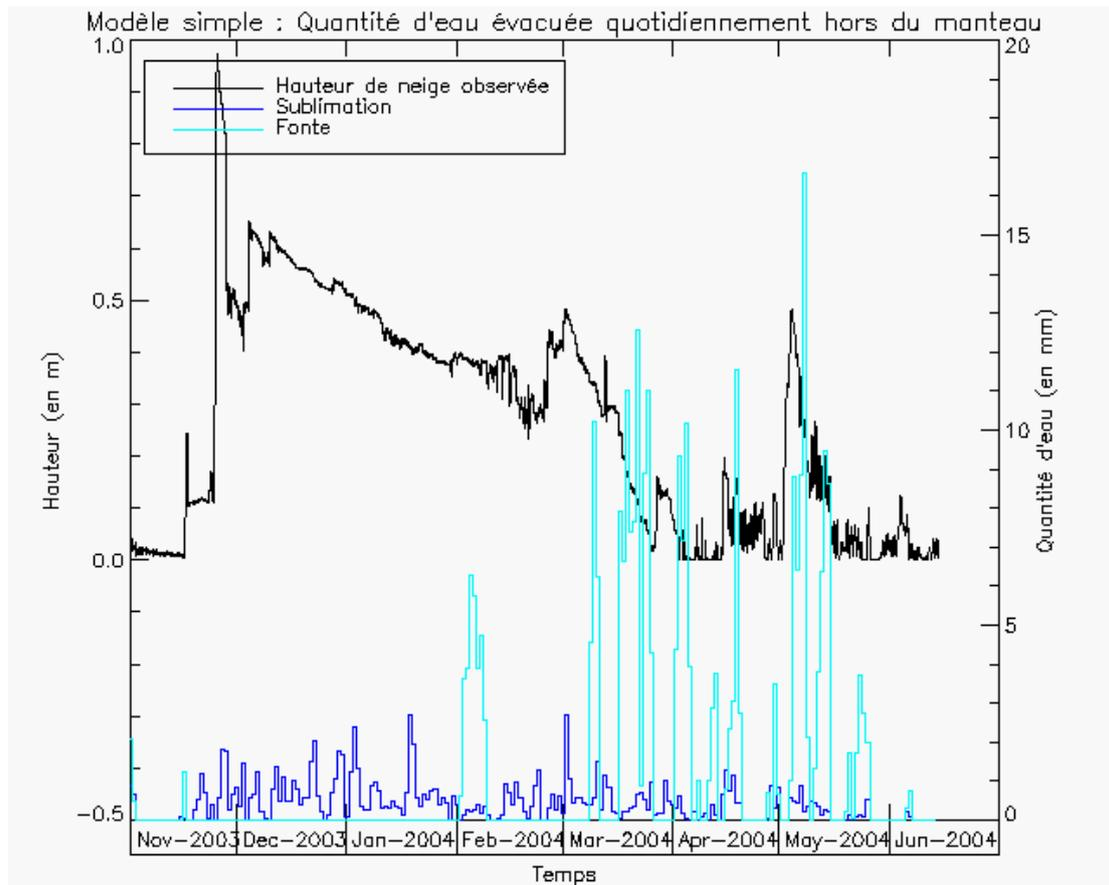
Figure 3: Observed snow height (black line), simulated sublimation (dark blue) and snowmelt (light blue) fluxes (mm/day) at the Oukaïmedem station in 2003-2004 (from Peltier, 2006)
