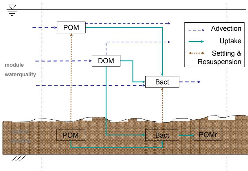
Figure 1: Scheme for processes of heterotrophic bacteria introduced in MOHID
