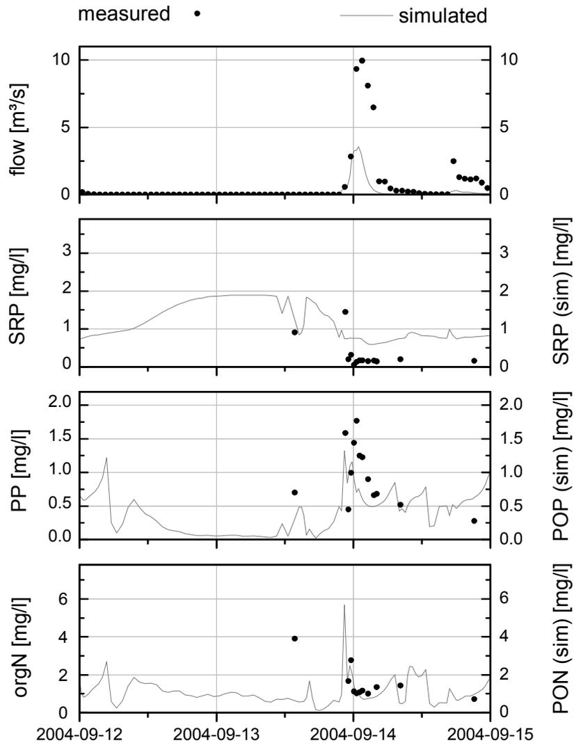
Figure 6: Measured and simulated concentrations at Sanglier (S) for 2004-09-13, Scenario “all” for inorganic phosphorus, particulate (organic) phosphorus and (particulate) organic nitrogen
