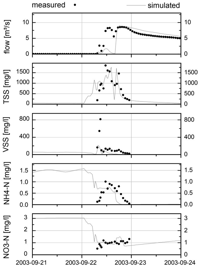
Figure 3: Measured and simulated concentrations at Sanglier (S) for 2003-09-22, Scenario “all” for particulates and dissolved inorganic nitrogen
