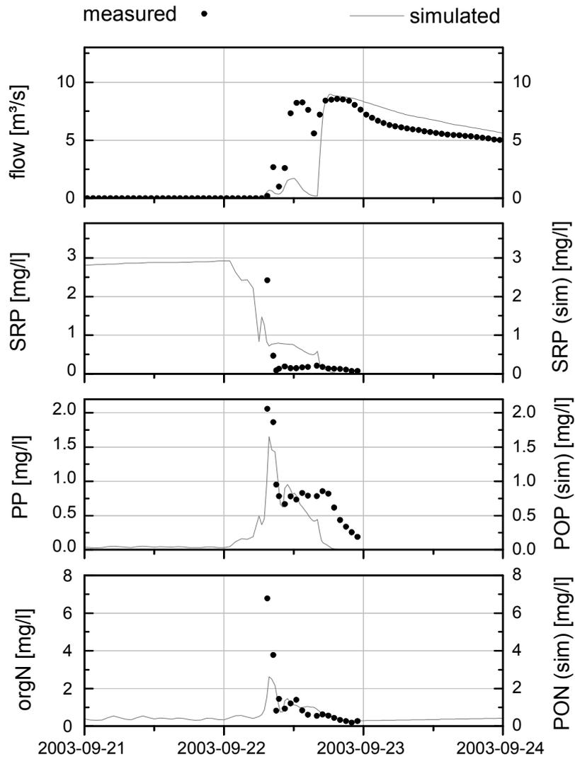
Figure 4: Measured and simulated concentrations at Sanglier (S) for 2003-09-22, Scenario “all” for inorganic phosphorus, particulate (organic) phosphorus and (particulate) organic nitrogen
