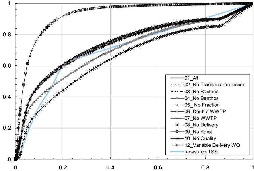
Figure 7: Comparison of normalized cumulative loads of measured TSS and all scenarios at S for 2003.09-22
