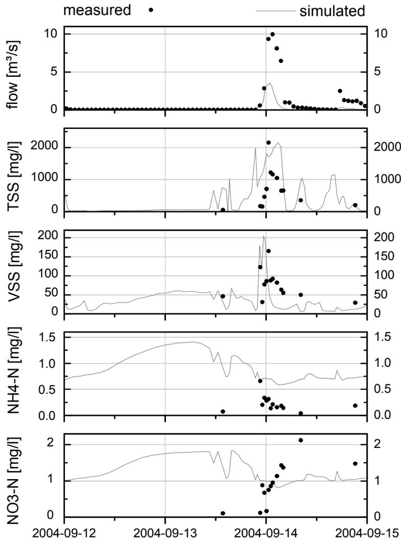
Figure 5: Measured and simulated concentrations at Sanglier (S) for 2004-09-13, Scenario “all” for particulates and dissolved inorganic nitrogen
