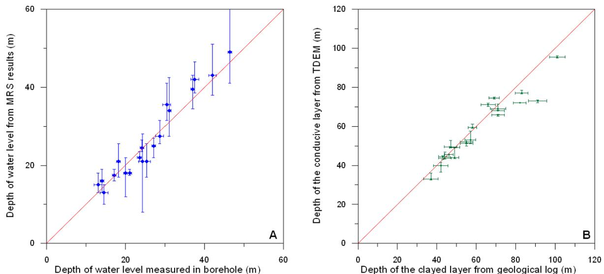
**Fig. 2: Comparison of the geometry of aquifer obtained by geophysical and by invasive methods. A. Water level. B. Bottom of aquifer.**
