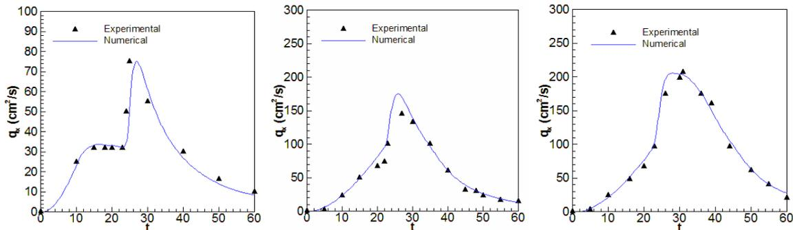
Figure 2. Numerical and experimental hydrograph for the 1D validation test. Case 1 (left), Case 2 (middle) and Case 3 (right).
