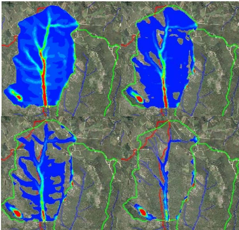
**Figure 10.** Sequence of drainage of the watershed at Esteiro, after the rainfall has finished.
