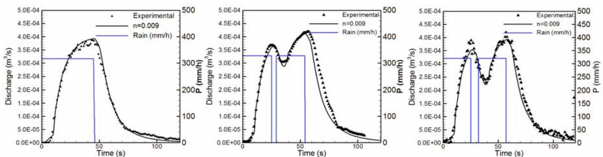
**Figure 7.** Numerical-experimental hydrographs for the 2D validation test. Case C1 (left), case C2 (middle) and case C3 (right).
