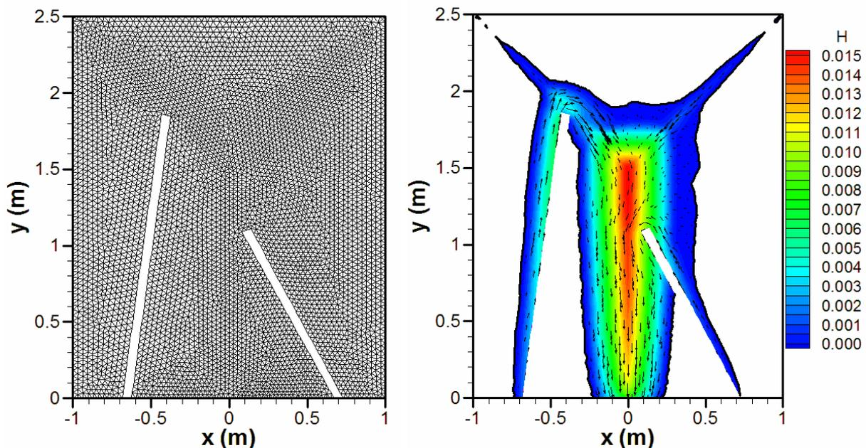
**Figure 6.** 2D Validation test. Case 1. Numerical mesh (left) and water depth and velocity field 5 seconds after the rain stops ( $T=50\text{s}$ ). Regions with water depth smaller than 0.1mm in white.
