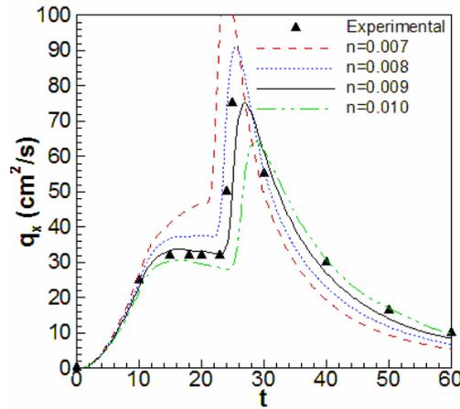
Figure 3. Sensitivity of the numerical results to the bed friction coefficient. 1D validation test. Case 1.
