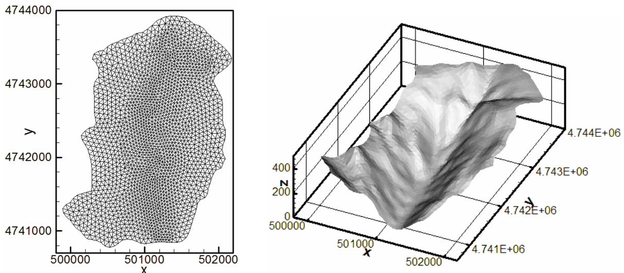
**Figure 8.** Numerical model of the watershed at Esteiro. Numerical mesh (left) and 3D view (right).
