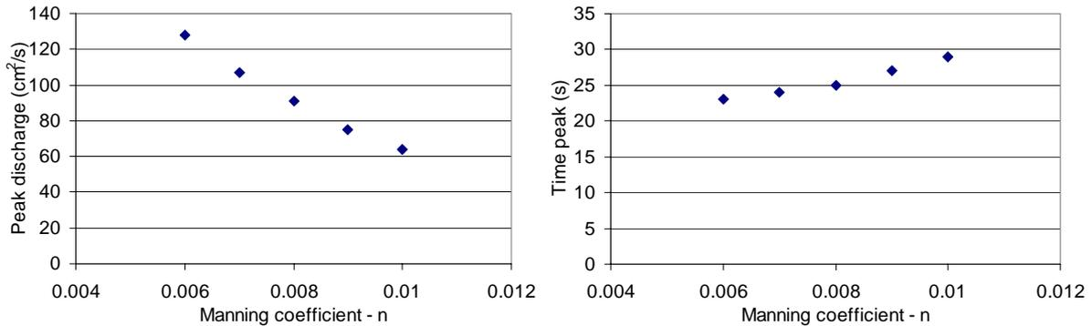
Figure 4. Sensitivity of the peak discharge to the bed friction coefficient. 1D validation test. Case 1.
