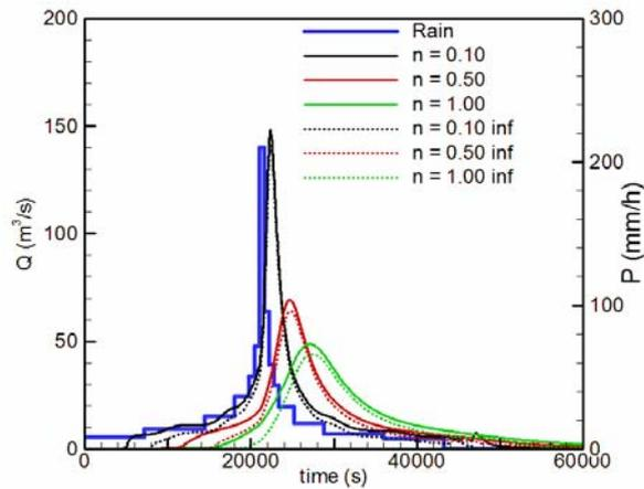
**Figure 9.** Hietogram for T=500 years, and hydrographs given by the numerical model for different bed friction coefficients, with infiltration and without infiltration.
