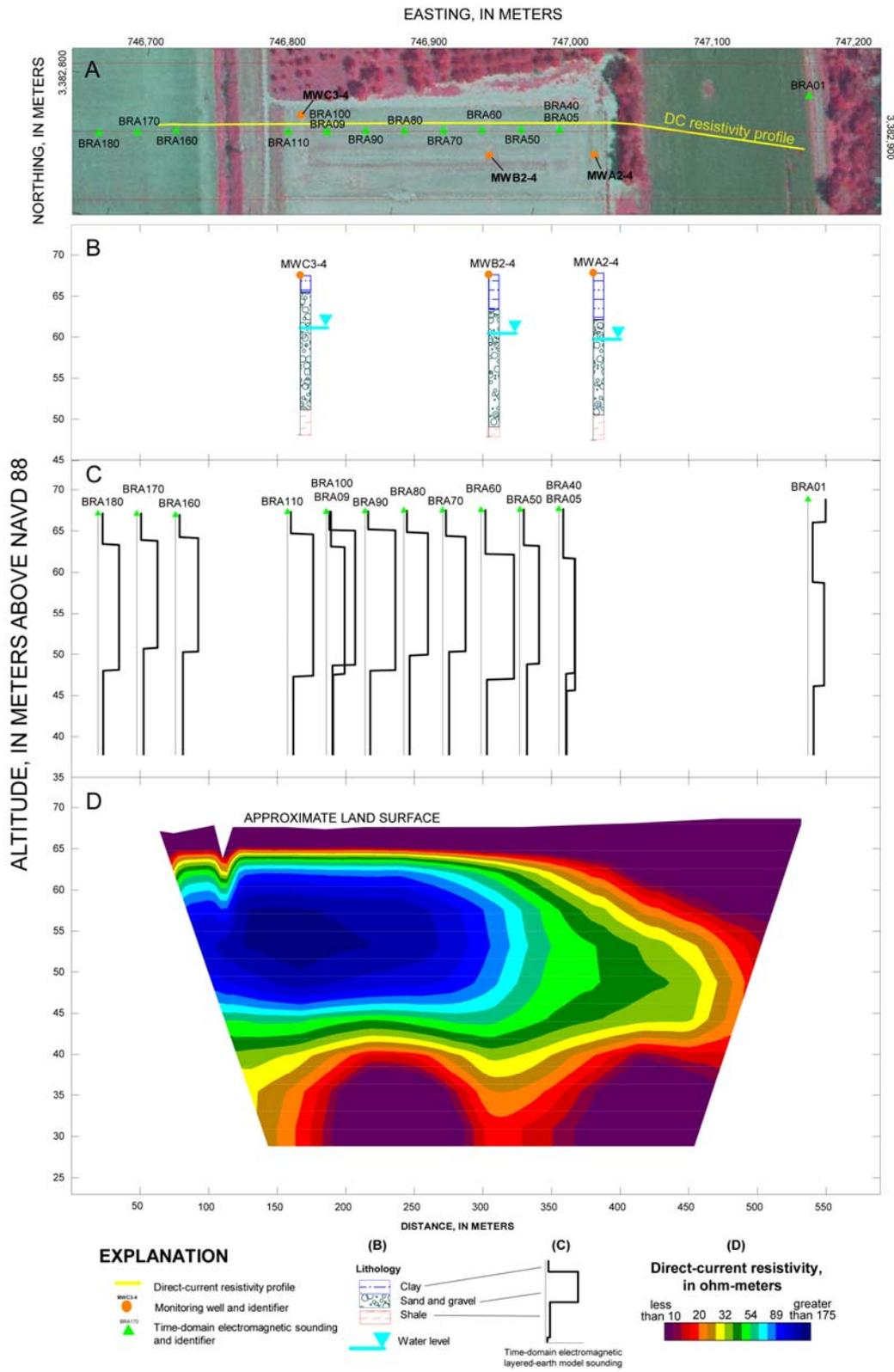
**Figure 5:** (A) Location of selected wells and time-domain electromagnetic (TDEM) soundings, (B) drillers' logs with static water level, (C) TDEM layered-earth model sounding results, and (D) robust inversion profile of two-dimensional direct-current dipole-dipole resistivity array, Brazos River Hydrologic Field Research Site, College Station, Texas.
