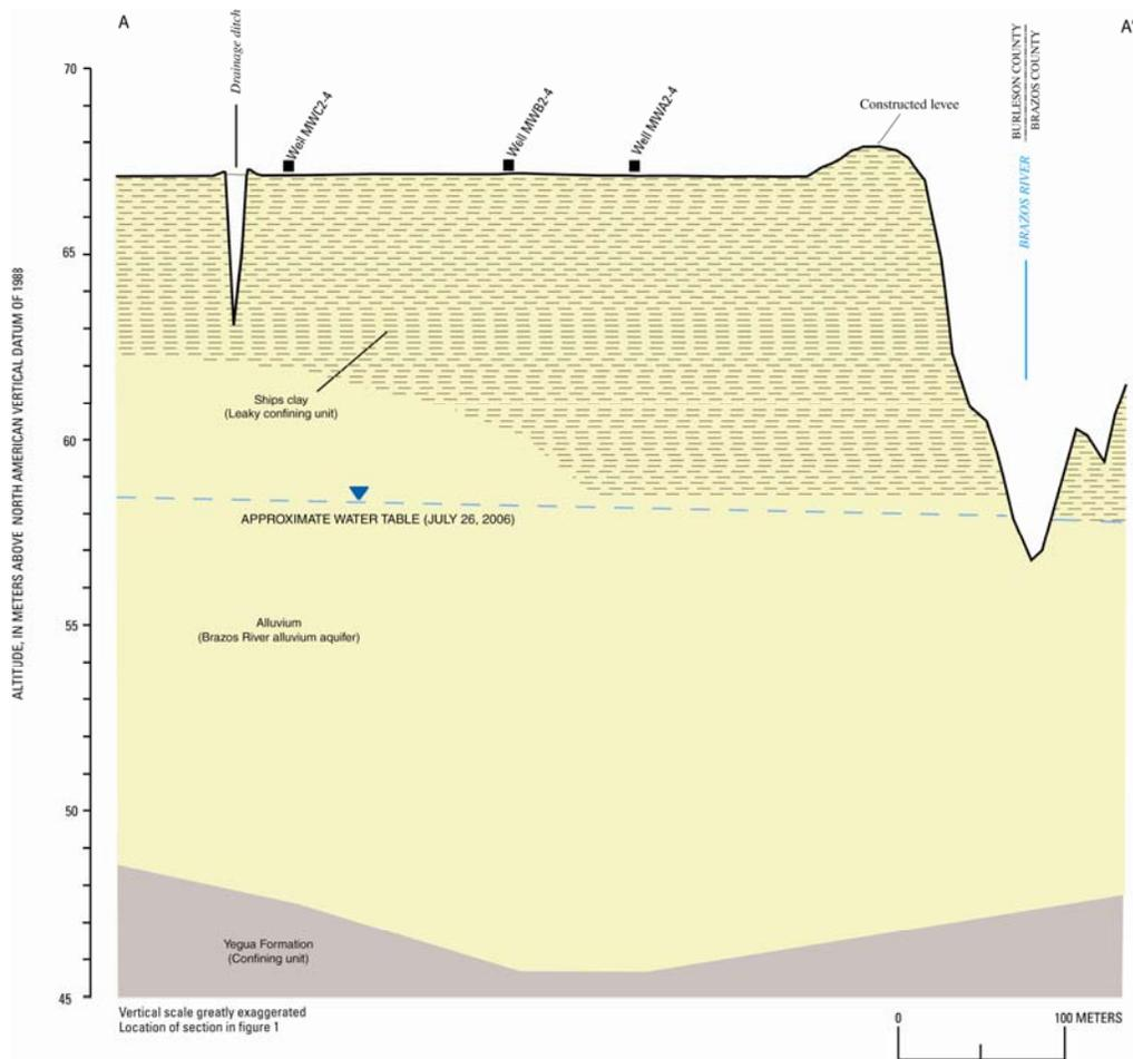
**Figure 2:** Conceptual hydrostratigraphic section A-A' across the Brazos River Hydrologic Field Research Site, College Station, Texas (modified from Wroblecki, 1996).
