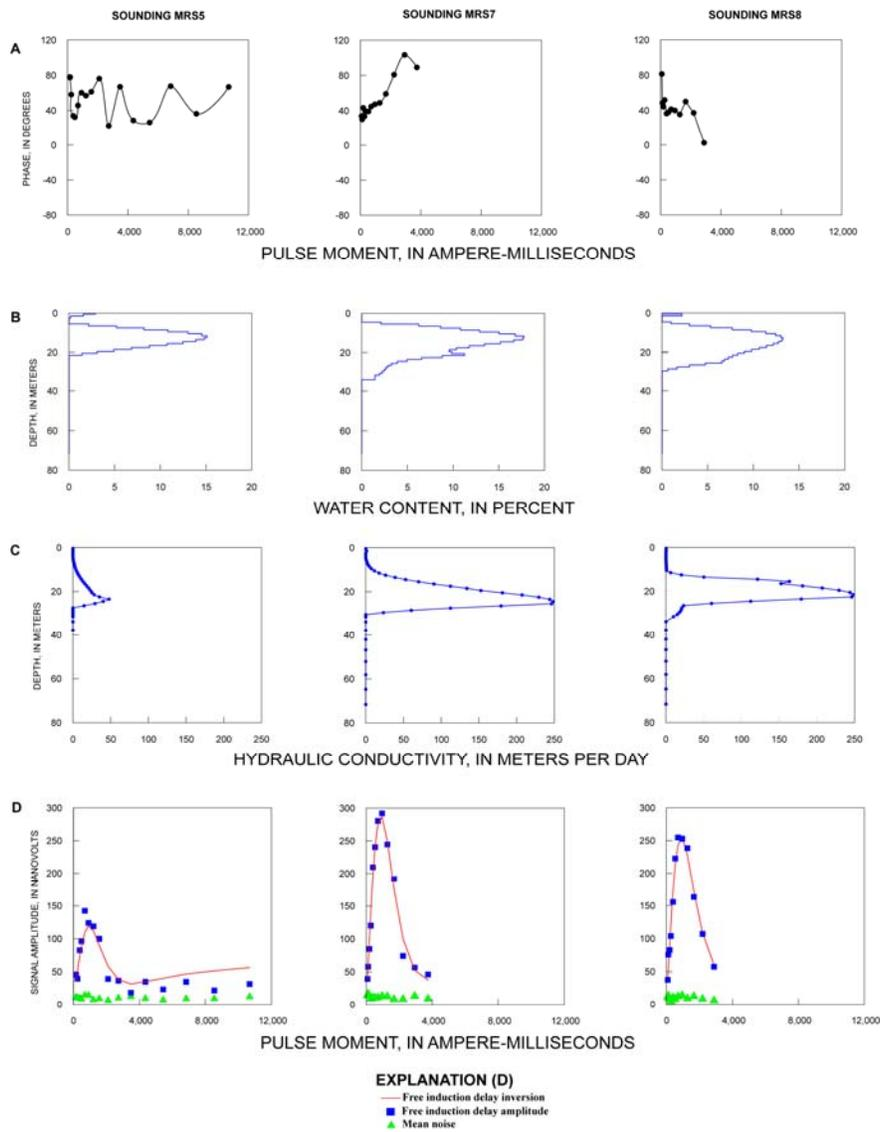
**Figure 3:** Magnetic resonance sounding (MRS) inversion results: (A) phase relative to pulse moment, (B) depth relative to water content, (C) depth relative to hydraulic conductivity, and (D) pulse moment relative to signal amplitude with signal-to-noise indication.
