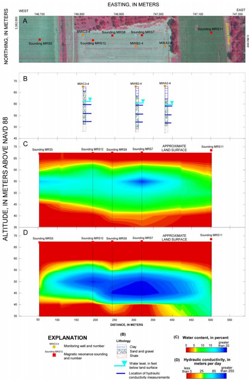
**Figure 6:** (A) Location of selected wells and magnetic resonance soundings (MRS), (B) drillers' logs with static water-level and locations of hydraulic conductivity measurements, (C) gridded percentage water content profile, and (D) gridded hydraulic conductivity profile based on MRS results, Brazos River Hydrologic Field Research Site, College Station, Texas.
