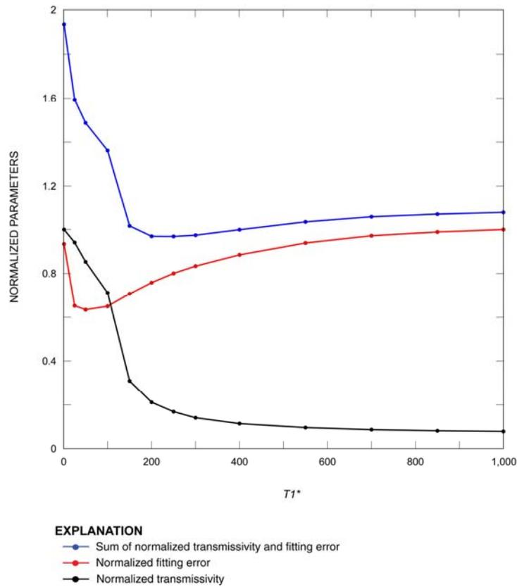
**Figure 4:** Calibration graph used to obtain the optimum relaxation time ( $T1^*$ ) for inversion of magnetic resonance sounding data using the default coefficient of permeability ( $Cp$ ) value of  $7.00 \times 10^{-9}$ , Brazos River Hydrologic Field Research Site, College Station, Texas.
