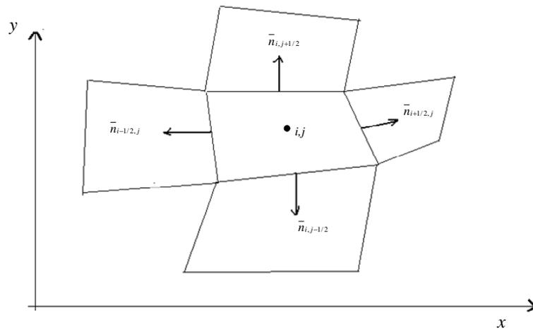
**Figure 2. Two-dimensional domain represented in finite volumes**
