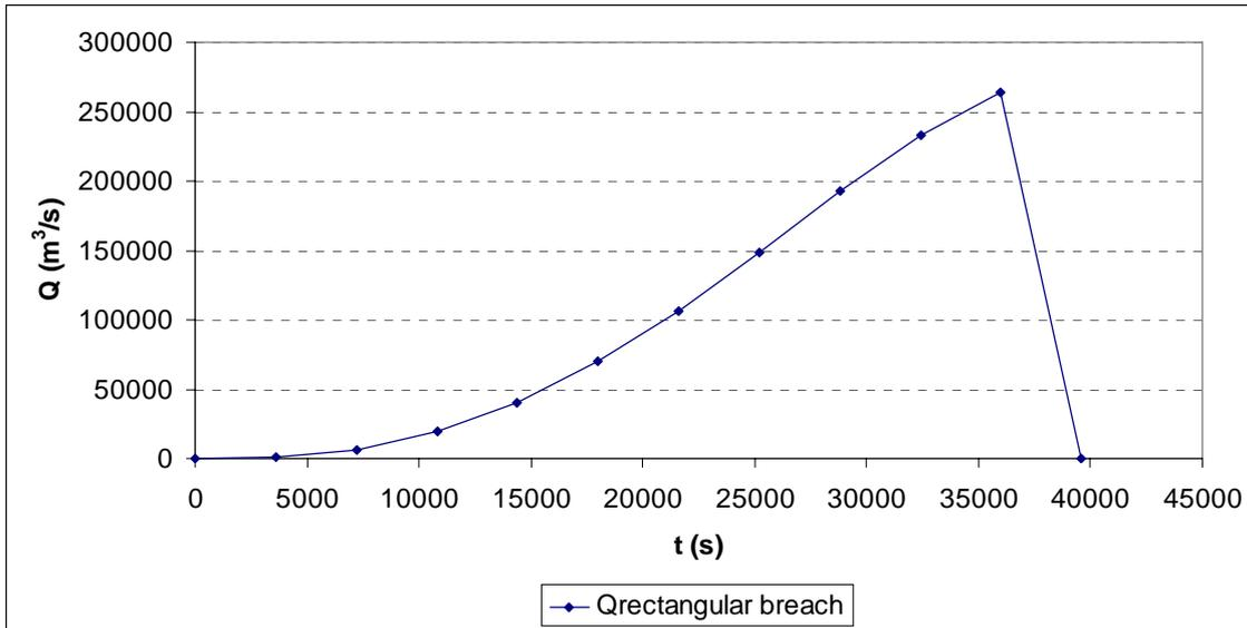
**Figure 5. Breach outlet hydrograph (assuming a rectangular shape)**
