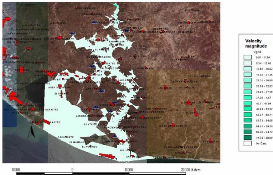
**Figure 8. Risk map of maximum water velocities. Dam break simulation of La Parota Dam, State of Guerrero, Mexico**
