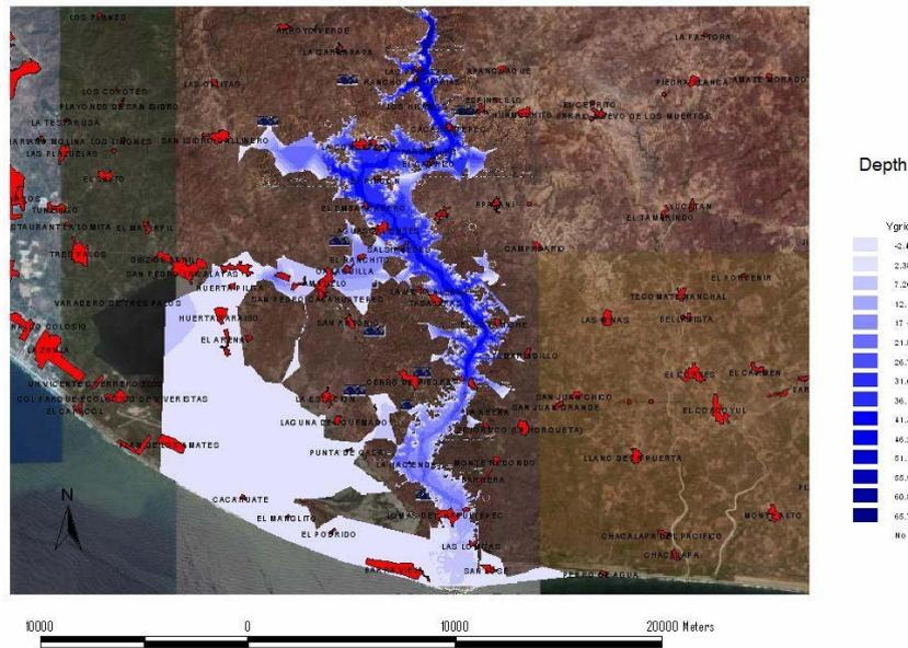
**Figure 7. Risk map of maximum water depths. Dam break simulation of La Parota Dam, State of Guerrero, Mexico**
