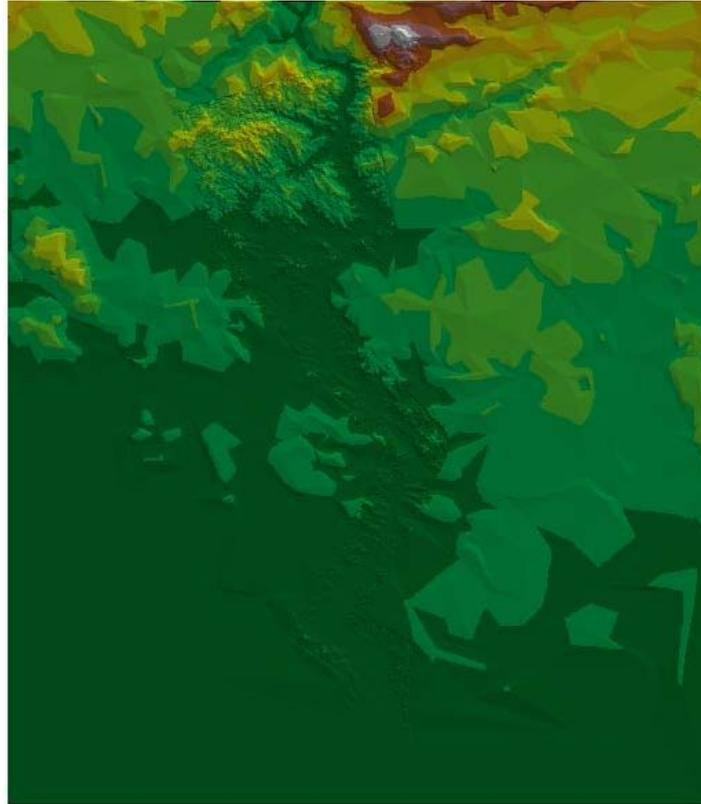
**Figure 3. Digital ground surface model (*tin* file, tol.  $\leq 0.5$  m)**
