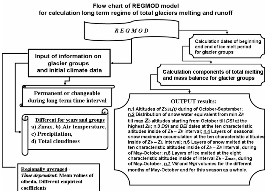
Fig. 2 Flow-chart of the REGMOD model.  $Z_{max}$  – is maximum altitude of snow line during ablation season,  $Z_{ssl}(t)$  – is seasonal snow line altitude on glacier surface at the moment  $t$ ,  $Z_e$  and  $Z_b$  – are consequently altitudes of the glacier's end and beginning,  $DSI$  and  $DEI$  are consequently dates of start and end of icemelt season.
