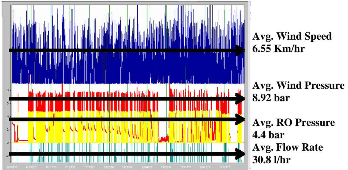
Figure No. 5 Average values of wind speed, wind pressure, RO pressure and flow rate during a 12 month eolic RO operating period.
