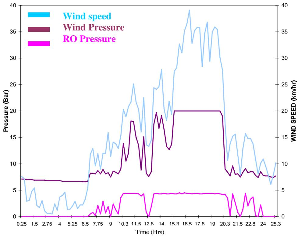
Figure No. 3 Wind speed, wind pressure and RO pressure during a 24 hr eolic reverse osmosis operating period.
