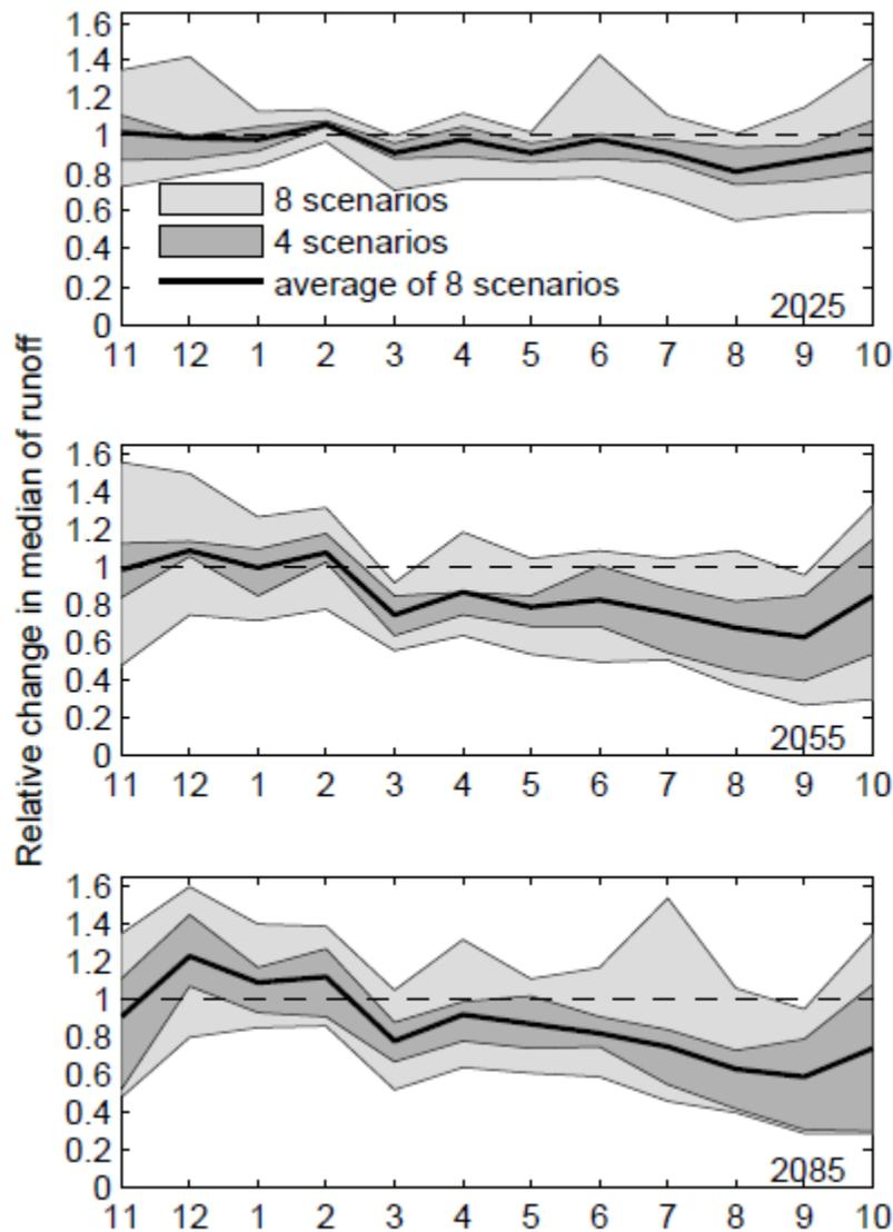
Fig. 2 Relative change in median of runoff for three time horizons with the range of uncertainty given by selecting a different climate change scenario for the closing profile of the Orlice River. The black line represents the average of all scenarios, the dark grey coloured area contains four scenarios and the light grey area is given by all of the scenarios.
