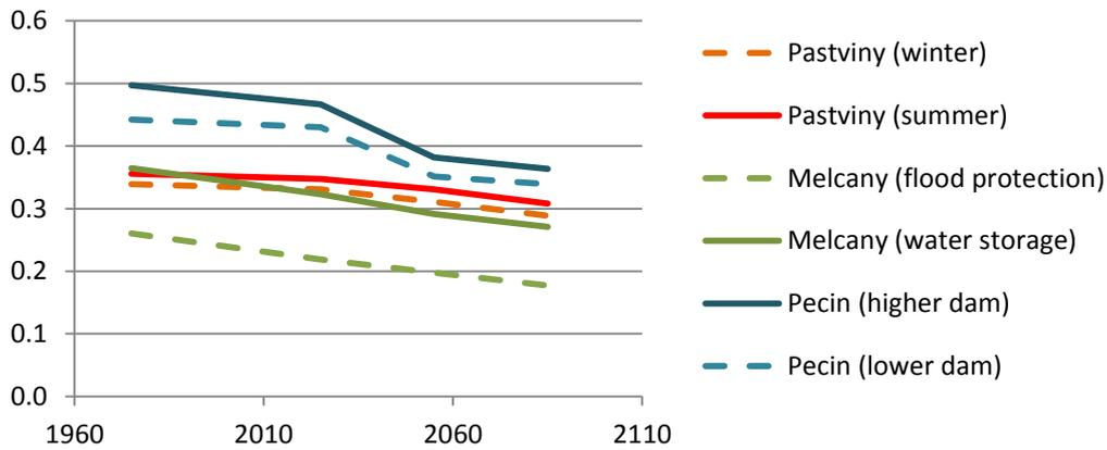
Fig. 4 The ratio between the total possible abstraction (security level 98.5 %) and the average discharge in the profile of the dam
