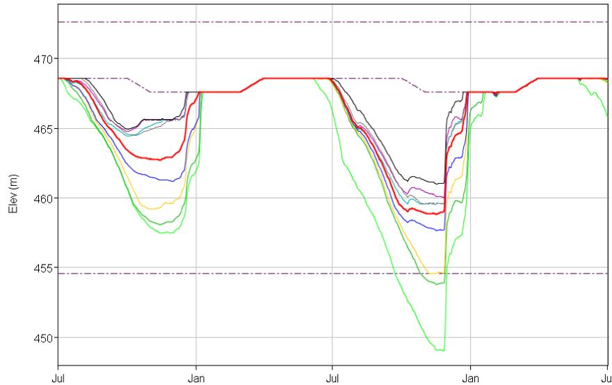
Fig. 3 Example of two year data of water levels in the Pastviny reservoir for the time horizon 2085 – simulated for increased water abstraction. The red line represents an average of all RCM simulations. Three scenarios indicate failure of the supply.
