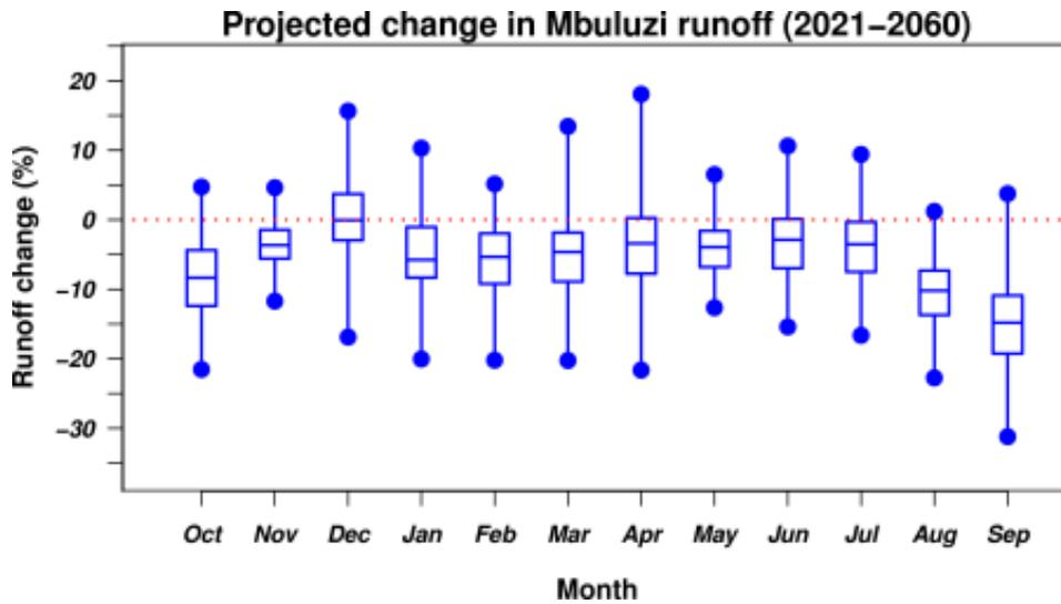
Figure10: Projected runoff change in the Mbuluzi catchment. The box plots show the 95% confidence interval extending from the circles, which show the 2.5% and 97.5% quantiles.
