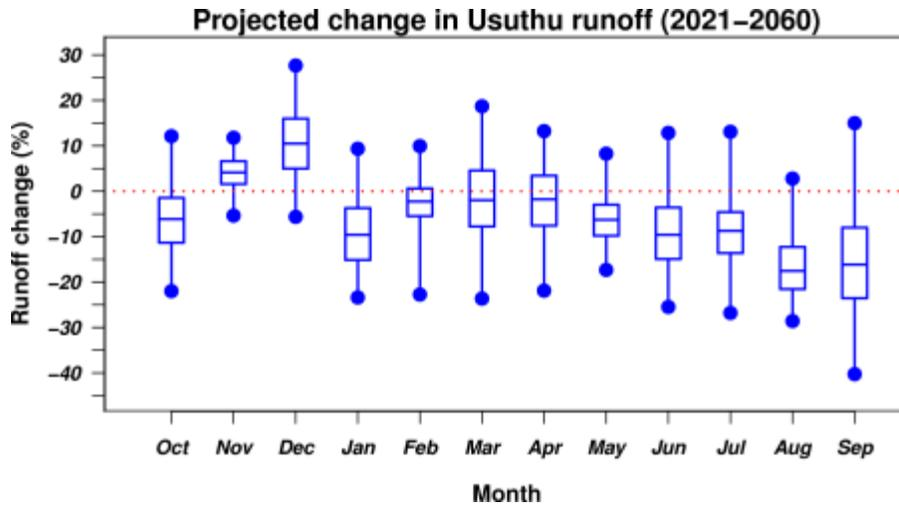
Figure 6: Projected runoff change in the Usuthu catchment. The box plots show the 95% confidence interval extending from the circles, which show the 2.5% and 97.5% quantiles.
