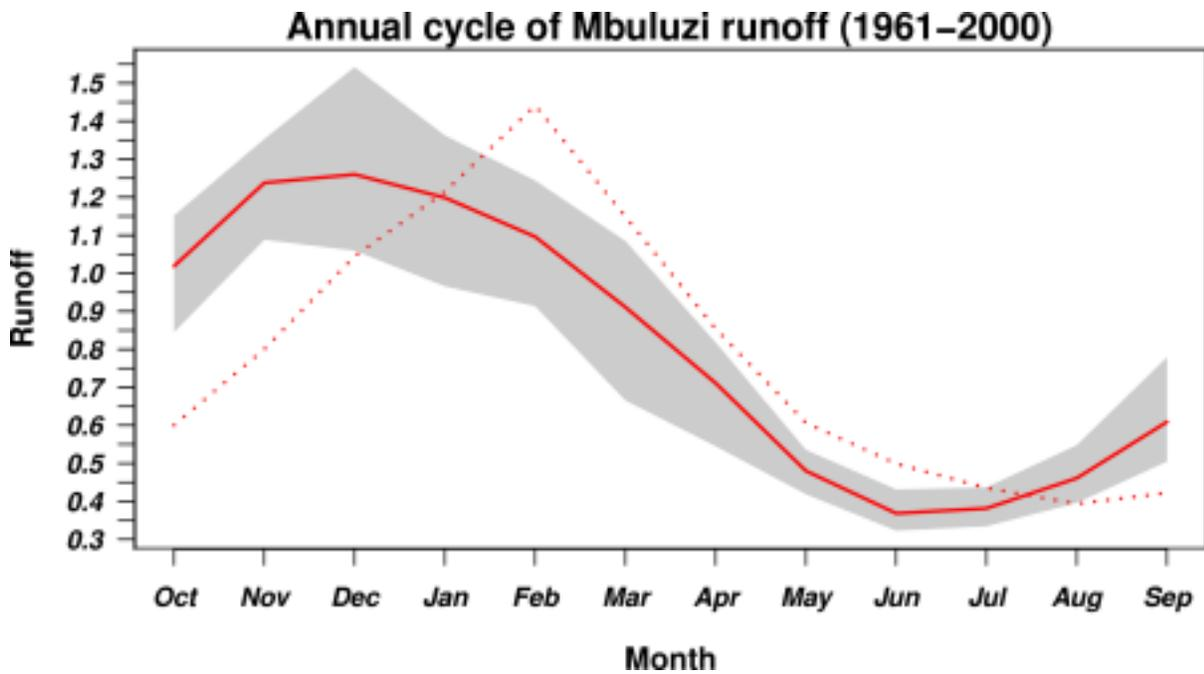
Figure 3. Observed and simulated streamflow in the Mbuluzi Catchment during verification
