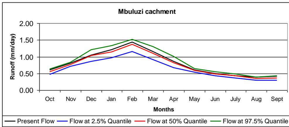
Figure 11: A comparison between present and future flows at the 2.5%, median, and the 97.5% quantiles runoff change in the Mbuluzi catchment
