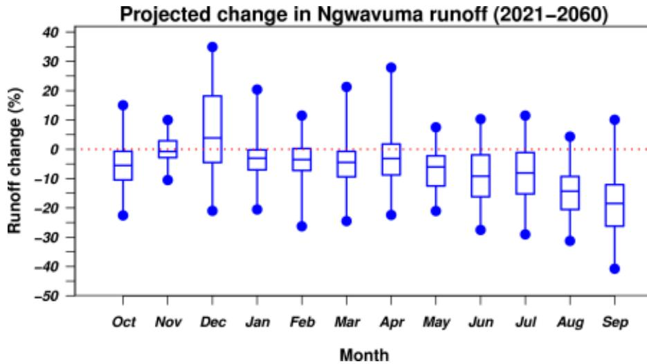
Figure12: Projected runoff change in the Ngwavuma catchment. The box plots show the 95% confidence interval extending from the circles, which show the 2.5% and 97.5% quantiles.
