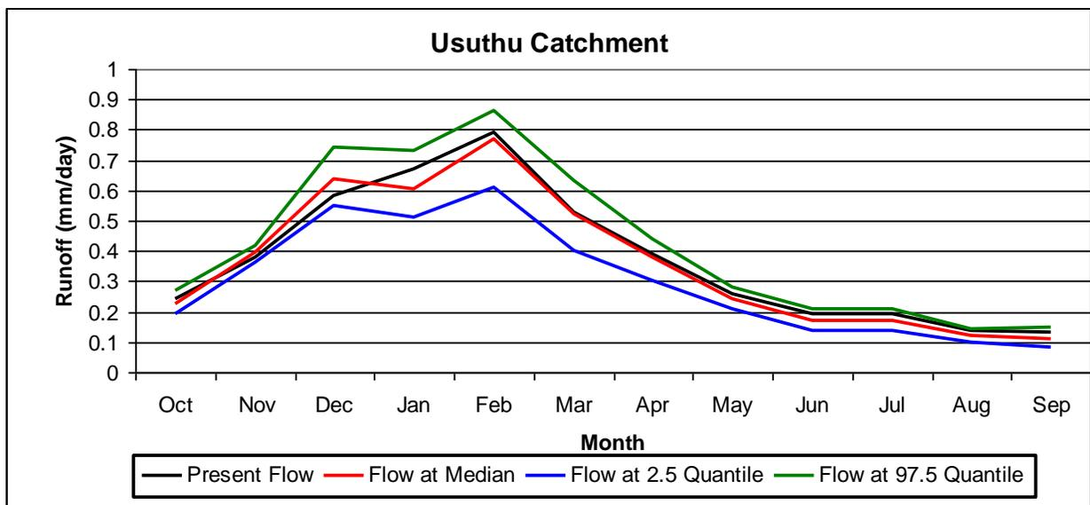
Figure 7: A comparison between present and future flows at the 2.5%, median, and 97.5% quantiles runoff change in the Usuthu catchment.
