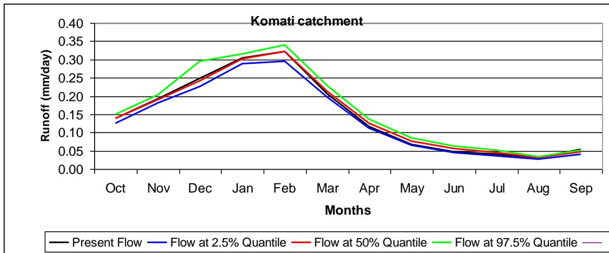
Figure 9: A comparison between present and future flows at the 2.5%, median, and the 97.5% quantiles runoff change in the Komati
