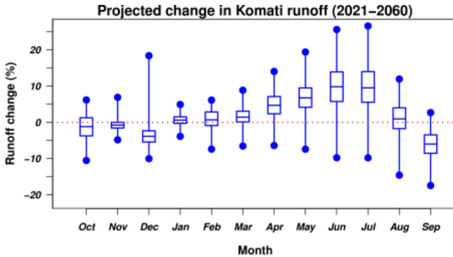
Figure 8: Projected runoff change in the Komati catchment. The box plots show the 95% confidence interval extending from the circles, which show the 2.5% and 97.5% quantiles.
