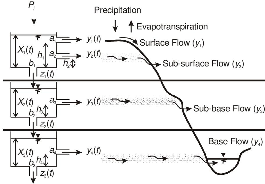
**Fig. 1** Schematic design tank model with three tanks.
