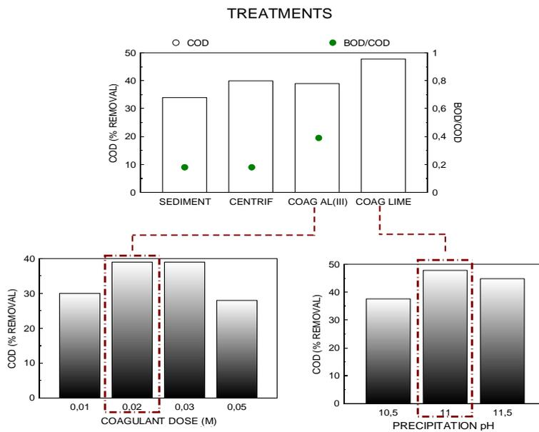
**Figure 1.** Influence of the pre-treatments in COD removal. Experimental conditions:  $pH_0=8, 3$ ;  $COD_0 =10, 4$  g/L.
