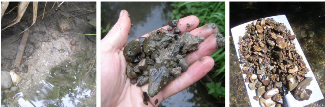
Figure 6: Complete colmation (left), medium colmation (manual sample, middle) and no colmation (shovel sample, right).
