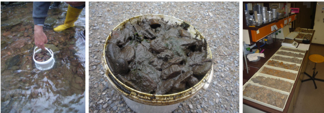
Figure 5. Sediment trap inserting, trap after three weeks exposure in river bed and grain-size analysis in laboratory.
