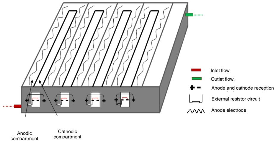
**Figure 1:** Schematic approach of 100lt MFC prototype reactor
