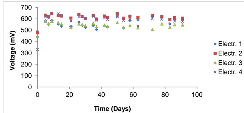
**Figure 2:** Open circuit voltage (OCV) generation from four electrode pairs in 100lt MFC
