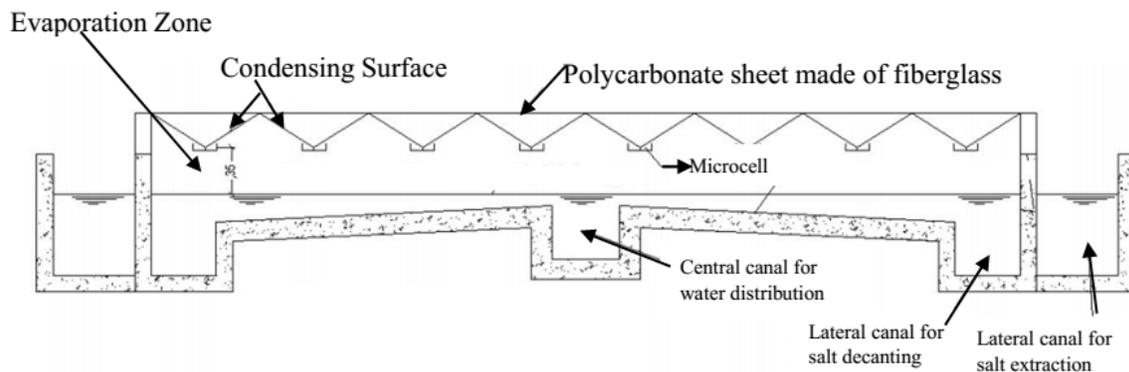
Figure 1. Cross section of the evaporation and condensation cells
