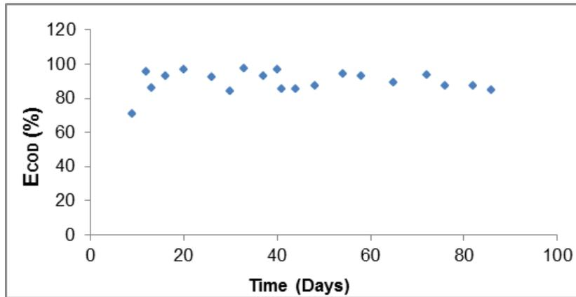
**Figure 7:**  $E_{\text{COD}}$ (%) from final MFC exit point
