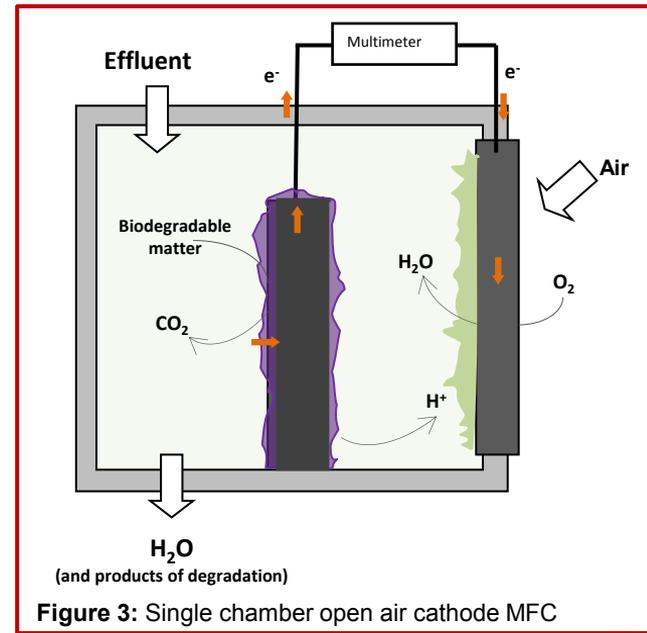
Figure 3: Single chamber open air cathode MFC
