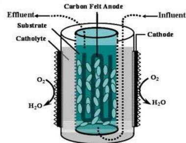
Figure 2: Tubular (vertical) MFC
