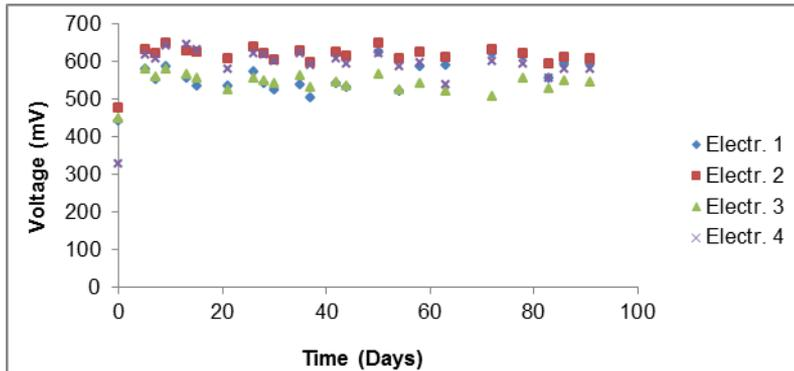
**Figure 6:** Open circuit voltage (OCV) generation from four electrode pairs in 100lt MFC
